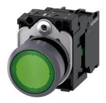
Illuminated pushbutton, 22 mm, round, plastic with metal front ring, green, pushbutton, flat, momentary contact type, with holder, 1NO, LED module with integrated LED 24 V AC/DC, screw terminal, with laser labeling, upper case and lower case, Always upper case at the beginning of the word
