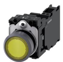
Illuminated pushbutton, 22 mm, round, plastic with metal front ring, yellow, pushbutton, flat, momentary contact type, with holder, 1 NO+1 NC, LED module with integrated LED 24 V AC/DC, spring-type terminal, Z=20-unit packaging
