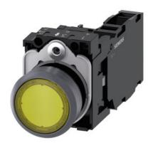
Illuminated pushbutton, 22 mm, round, plastic with metal front ring, yellow, pushbutton, flat, momentary contact type, with holder, 1 NO+1 NC, LED module with integrated LED 24 V AC/DC, screw terminal, with laser labeling, upper case
