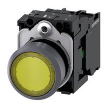
Illuminated pushbutton, 22 mm, round, plastic with metal front ring, yellow, pushbutton, flat, momentary contact type, with holder, 1NO, LED module with integrated LED 24 V AC/DC, screw terminal, with laser labeling, upper case
