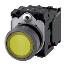
Illuminated pushbutton, 22 mm, round, plastic with metal front ring, yellow, pushbutton, flat, momentary contact type, with holder, 1NO, LED module with integrated LED 24 V AC/DC, screw terminal, with laser labeling, upper case and lower case, always upper case at beginning of line
