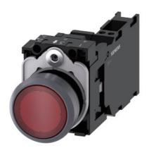
Illuminated pushbutton, 22 mm, round, plastic with metal front ring, red, pushbutton, flat, momentary contact type, with holder, 1 NO+1 NC, LED module with integrated LED 24 V AC/DC, spring-type terminal, with laser labeling, upper case and lower case, Always upper case at the beginning of the word
