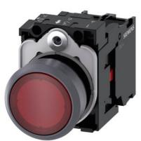
Illuminated pushbutton, 22 mm, round, plastic with metal front ring, red, pushbutton, flat, momentary contact type, with holder, 1NC, LED module with integrated LED 24 V AC/DC, screw terminal, with laser labeling, lower case
