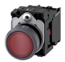
Illuminated pushbutton, 22 mm, round, plastic with metal front ring, red, pushbutton, flat, momentary contact type, with holder, 1NC, LED module with integrated LED 24 V AC/DC, screw terminal, with laser labeling, upper case
