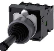
Coordinate switch, 22 mm, round, plastic with metal front ring, black, 4 switch positions, momentary contact type, with mechanical interlocking in O position, with holder, 1 NO, 1 NO, 1 NO, screw terminal
