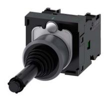
Coordinate switch, 22 mm, round, plastic with metal front ring, black, 2 switch positions, vertical, momentary contact type, with mechanical interlocking in O position, with holder, 1 NO, 1 NO, screw terminal, with laser labeling, upper case and lower case, always upper case at the beginning of the word
