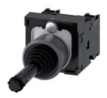
Coordinate switch, 22 mm, round, plastic with metal front ring, black, 2 switch positions, vertical, momentary contact type, with mechanical interlocking in O position, with holder, 1 NO, 1 NO, screw terminal, with laser labeling, upper case and lower case, always upper case at beginning of line
