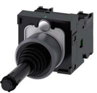
Coordinate switch, 22 mm, round, plastic with metal front ring, black, 2 switch positions, horizontal, momentary contact type, with mechanical interlocking in O position, with holder, 1 NO, 1 NO, screw terminal
