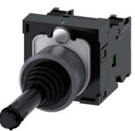
Coordinate switch, 22 mm, round, plastic with metal front ring, black, 2 switch positions, horizontal, momentary contact type, with mechanical interlocking in O position, with holder, 1 NO, 1 NO, screw terminal, with laser labeling, lower case
