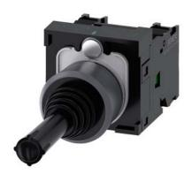
Coordinate switch, 22 mm, round, plastic with metal front ring, black, 2 switch positions, vertical latching, without mechanical interlocking, in O position, with holder, 1 NO, 1 NO, screw terminal, with laser labeling, upper case
