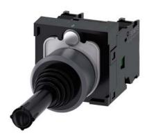
Coordinate switch, 22 mm, round, plastic with metal front ring, black, 2 switch positions, horizontal latching, without mechanical interlocking, in O position, with holder, 1 NO, 1 NO, screw terminal, with laser labeling, inscription or symbol, Customer-specific selection with SIRIUS ACT configurator (CIN)
