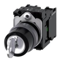
RONIS key-operated switch, 22 mm, round, plastic with metal front ring, lock number SB30, with 2 keys, 3 switch positions I-O-II, latching, actuating angle 2x45°, 10:30h/12h/13:30h, Key removal I+O+II, with holder, 1 NO, 1 NO, screw terminal, possible special locks: SB31, 421, 455, with laser labeling, upper case and lower case, always upper case at the beginning of the word
