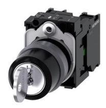
RONIS key-operated switch, 22 mm, round, plastic with metal front ring, lock number SB30, with 2 keys, 3 switch positions I-O-II, latching, actuating angle 2x45°, 10:30h/12h/13:30h, Key removal I+O+II, with holder, 1 NO, 1 NO, screw terminal, Z=20-unit packaging
