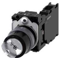
RONIS keyswitch, 22 mm, round, plastic with metal front ring, Lock number SB30, with 2 keys, 2 switch positions O-I, latching, 10:30/1:30 o'clock, key removal O+I, with holder, 1 NO+1 NC, spring-type terminal, possible special locks: SB31, 421, 455
