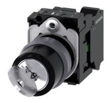
RONIS key-operated switch, 22 mm, round, plastic with metal front ring, lock number SB30, with 2 keys, 2 switch positions O-I, latching, actuating angle 90°, 10:30h/13:30h, key removal O+I, with holder, 1 NO, Spring-type terminal
