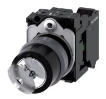
RONIS key-operated switch, 22 mm, round, plastic with metal front ring, lock number SB30, with 2 keys, 2 switch positions O-I, latching, actuating angle 90°, 10:30h/13:30h, key removal O+I, with holder, 1 NO, spring-type terminal, possible special locks: SB31, 421, 455, with laser labeling, inscription or symbol Customer-specific selection with SIRIUS ACT configurator (CIN)
