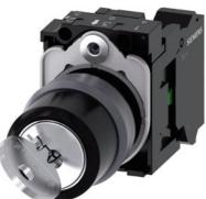
RONIS key-operated switch, 22 mm, round, plastic with metal front ring, lock number SB30, with 2 keys, 2 switch positions O-I, latching, actuating angle 90°, 10:30h/13:30h, key removal O+I, with holder, 1 NO, spring-type terminal, possible special locks: SB31, 421, 455, with laser labeling, upper case and lower case, always upper case at the beginning of the word
