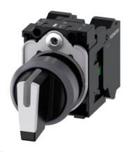
Selector switch, illuminable, 22 mm, round, plastic with metal front ring, white, selector switch, short, 3 switch positions I>O<II, momentary contact type, actuating angle  $2x45^{\circ}$ , 10:30h/12h/13:30h, with holder, 1 NO, 1 NO, Spring-type terminal
