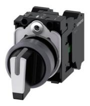
Selector switch, illuminable, 22 mm, round, plastic with metal front ring, white, selector switch, short, 3 switch positions I>O<II, momentary contact type, actuating angle 2x45°, 10:30h/12h/13:30h, with holder, 1 NO, 1 NO, spring-type terminal, with laser labeling, upper case and lower case, always upper case at the beginning of the word
