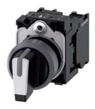
Selector switch, illuminable, 22 mm, round, plastic with metal front ring, white, selector switch, short, 3 switch positions I>O<II, momentary contact type, actuating angle 2x45°, 10:30h/12h/13:30h, with holder, 1 NO, 1 NO, screw terminal, with laser labeling, upper case and lower case, always upper case at the beginning of the word
