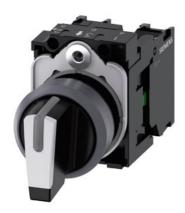
Selector switch, illuminable, 22 mm, round, plastic with metal front ring, white, selector switch, short, 3 switch positions I>O<II, momentary contact type, actuating angle 2x45°, 10:30h/12h/13:30h, with holder, 1 NO, 1 NO, screw terminal, with laser labeling, upper case and lower case, always upper case at beginning of line
