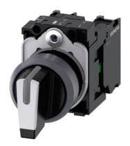
Selector switch, illuminable, 22 mm, round, plastic with metal front ring, white, selector switch, short, 3 switch positions I-O-II, latching, actuating angle 2x45°, 10:30h/12h/13:30h, with holder, 1 NO, 1 NO, screw terminal, with laser labeling, lower case
