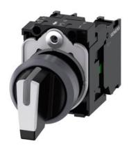
Selector switch, illuminable, 22 mm, round, plastic with metal front ring, white, selector switch, short, 3 switch positions I-O-II, latching, actuating angle 2x45°, 10:30h/12h/13:30h, with holder, 1 NO, 1 NO, screw terminal, with laser labeling, upper case
