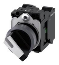
Selector switch, illuminable, 22 mm, round, plastic with metal front ring, white, selector switch, short, 2 switch positions O-I, latching, actuating angle 90°, 10:30h/13:30h, with holder, 1 NO, 1 NC, spring-type terminal, with laser labeling, upper case and lower case, always upper case at beginning of line
