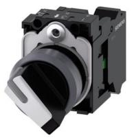
Selector switch, illuminable, 22 mm, round, plastic with metal front ring, white, selector switch, short, 2 switch positions O-I, latching, actuating angle 90°, 10:30h/13:30h, with holder, 1 NO, spring-type terminal, with laser labeling, upper case and lower case, always upper case at the beginning of the word
