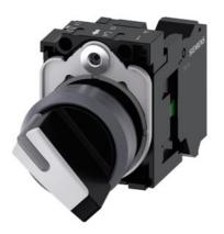
Selector switch, illuminable, 22 mm, round, plastic with metal front ring, white, selector switch, short, 2 switch positions O-I, latching, actuating angle 90°, 10:30h/13:30h, with holder, 1 NO, spring-type terminal, with laser labeling, lower case
