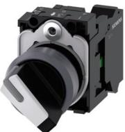
Selector switch, illuminable, 22 mm, round, plastic with metal front ring, white, selector switch, short, 2 switch positions O-I, latching, actuating angle 90°, 10:30h/13:30h, with holder, 1 NO, spring-type terminal, Z=20-unit packaging
