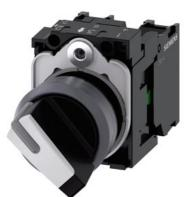
Selector switch, illuminable, 22 mm, round, plastic with metal front ring, white, selector switch, short, 2 switch positions O-I, latching, actuating angle 90°, 10:30h/13:30h, with holder, 1 NO, 1 NC, screw terminal, with laser labeling, inscription or symbol Customer-specific selection with SIRIUS ACT configurator (CIN)
