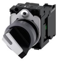
Selector switch, illuminable, 22 mm, round, plastic with metal front ring, white, selector switch, short, 2 switch positions O-I, latching, actuating angle 90°, 10:30h/13:30h, with holder, 1 NO, screw terminal, with laser labeling, lower case
