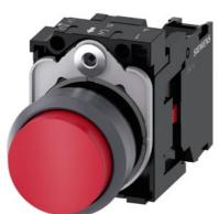
Pushbutton, 22 mm, round, plastic with metal front ring, red, pushbutton, raised, momentary contact type, with holder, 1 NC, screw terminal
