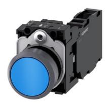
Pushbutton, 22 mm, round, plastic with metal front ring, blue, pushbutton, flat, momentary contact type, with holder, 1 NO+1 NC, screw terminal, with laser labeling, inscription or symbol Customer-specific selection with SIRIUS ACT configurator (CIN)
