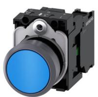
Pushbutton, 22 mm, round, plastic with metal front ring, blue, pushbutton, flat, momentary contact type, with holder, 1 NO, screw terminal, Z=20-unit packaging
