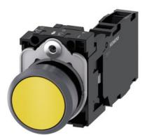
Pushbutton, 22 mm, round, plastic with metal front ring, yellow, pushbutton, flat, momentary contact type, with holder, 1 NO+1 NC, screw terminal, with laser labeling, upper case and lower case, always upper case at the beginning of the word
