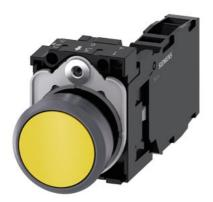
Pushbutton, 22 mm, round, plastic with metal front ring, yellow, pushbutton, flat, momentary contact type, with holder, 1 NO+1 NC, screw terminal, with laser labeling, upper case and lower case, always upper case at beginning of line
