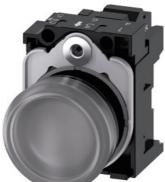
Indicator lights, 22 mm, round, plastic, clear, lens, smooth, with holder, LED module, with integrated LED 230 V AC, spring-type terminal, Z=20-unit packaging
