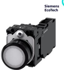
Illuminated pushbutton, 22 mm, round, plastic, white, pushbutton, flat, momentary contact type, with holder, 1 NO+1 NC, LED module with integrated LED 230 V AC, screw terminal, with laser labeling, lower case
