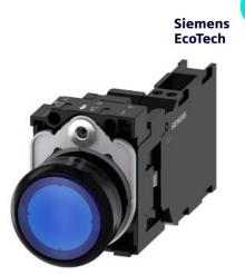
Illuminated pushbutton, 22 mm, round, plastic, blue, pushbutton, flat, momentary contact type, with holder, 1 NO+1 NC, LED module with integrated LED 230 V AC, spring-type terminal, with laser labeling, lower case
