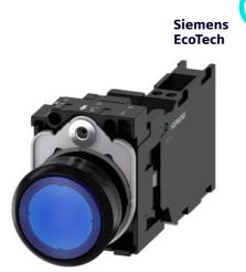
Illuminated pushbutton, 22 mm, round, plastic, blue, pushbutton, flat, momentary contact type, with holder, 1 NO+1 NC, LED module with integrated LED 230 V AC, spring-type terminal, with laser labeling, upper case and lower case, always upper case at beginning of line
