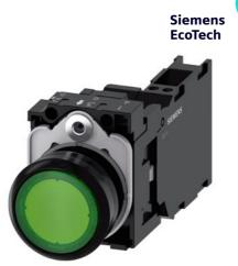
Illuminated pushbutton, 22 mm, round, plastic, green, pushbutton, flat, momentary contact type, with holder, 1 NO+1 NC, LED module with integrated LED 230 V AC, spring-type terminal, with laser labeling, lower case
