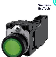
Illuminated pushbutton, 22 mm, round, plastic, green, pushbutton, flat, momentary contact type, with holder, 1 NO+1 NC, LED module with integrated LED 230 V AC, screw terminal, with laser labeling, symbol number according to, ISO 7000 or IEC 60417
