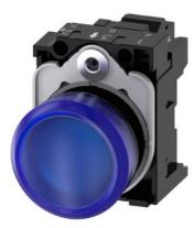
Indicator lights, 22 mm, round, plastic, blue, lens, smooth, with holder, LED module, with integrated LED 110 V AC, spring-type terminal, with laser labeling, inscription or symbol Customer-specific selection with SIRIUS ACT configurator (CIN)
