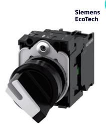
Selector switch, illuminable, 22 mm, round, plastic, white, selector switch, short, 2 switch positions O-I, latching, 10:30h/13:30h, with holder, with LED module, with integrated LED 110 V AC, 1 NO, screw terminal
