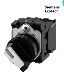
Selector switch, illuminable, 22 mm, round, plastic, white, selector switch, short, 2 switch positions O-I, latching, 10:30h/13:30h, with holder, with LED module, with integrated LED 110 V AC, 1 NO, screw terminal, with laser labeling, upper case and lower case, always upper case at the beginning of the word
