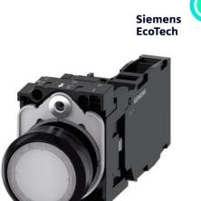
Illuminated pushbutton, 22 mm, round, plastic, white, pushbutton, flat, momentary contact type, with holder, 1 NO+1 NC, LED module with integrated LED 110 V AC, screw terminal, with laser labeling, symbol number according to, ISO 7000 or IEC 60417
