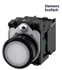
Illuminated pushbutton, 22 mm, round, plastic, white, pushbutton, flat, momentary contact type, with holder, 1NO, LED module with integrated LED 110 V AC, screw terminal, with laser labeling, lower case
