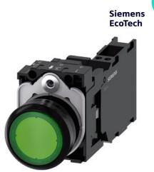
Illuminated pushbutton, 22 mm, round, plastic, green, pushbutton, flat, momentary contact type, with holder, 1 NO+1 NC, LED module with integrated LED 110 V AC, spring-type terminal, with laser labeling, inscription or symbol Customer-specific selection with SIRIUS ACT configurator (CIN)
